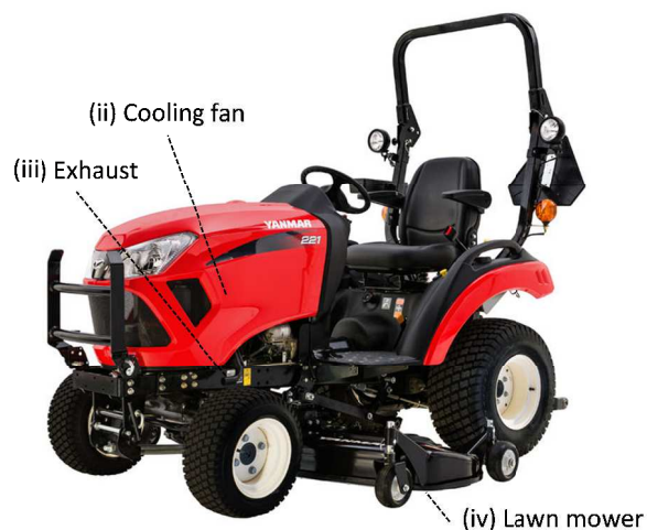
Fig. 4-1 Flow induced noise emitted from a tractor
