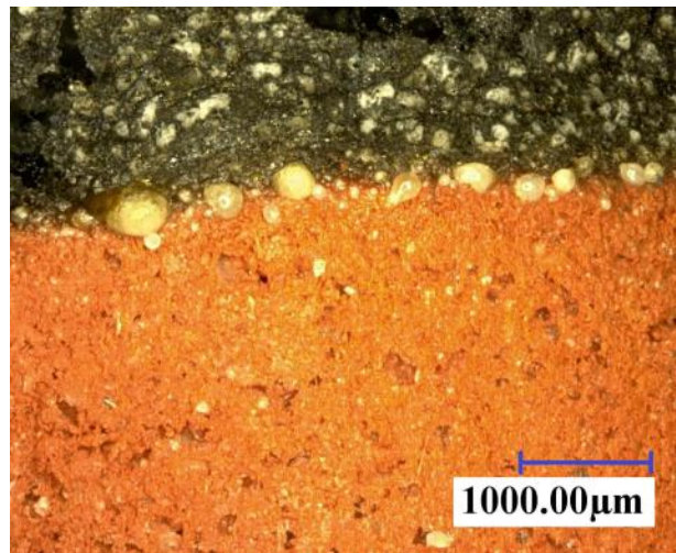
Fig.3-17 DMS photograph of the burned surface of quenched AN/Fe 2 O 3 propellant at \xi=4\% .
